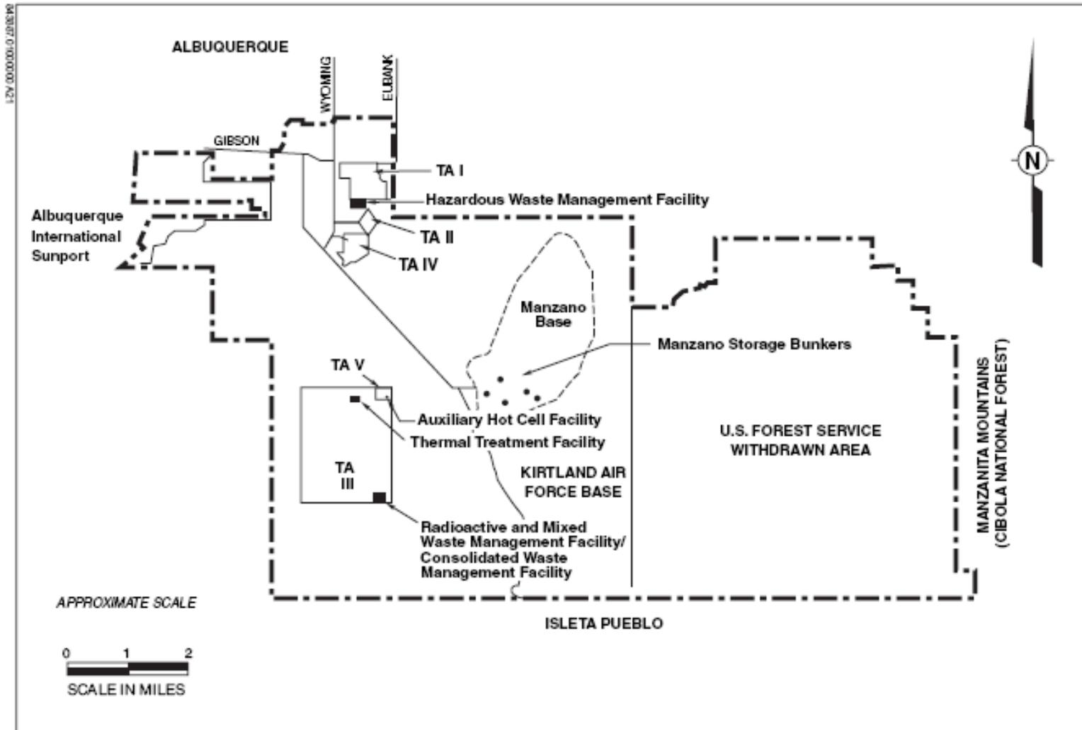
**Hazardous Waste Management Facility (HWMF).** The HWMF is south of SNL/NM TA-I. used for storage and packaging of RCRA-regulated wastes. The wastes are transported to off-site RCRA-permitted facilities for treatment, storage, and/or disposal.
